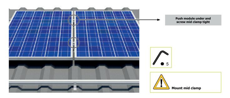
Ensure that the mid clamp clamps both module frames at the clamping area defined by the module manufacturer.
