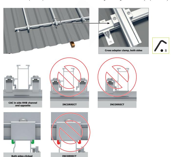
Depending on the structural requirements of the location and the installation situation, several cross adapter clamps may be required per crossing point. If a second cross adapter clamp is required, it is fixed to the opposite side, as described above (torque 8-10 Nm).
