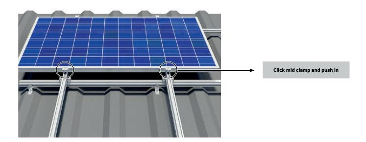
Now push the next module under the mid clamp, adjust the mid clamp to the height of the module frame and tighten the screw (torque 8-10 Nm).
